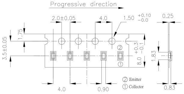
Unit: mm Tolerance: ±0.1mm
